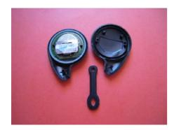
Remote key cases are made of simple plastic and they are prone to breakage especially around the key ring loop. In most cases the key ring loop is the first to give. Majority of the keyring loops are not exchangeable. Fortunately some loops are made separate to the plastic shell and can be replaced with no problem at all. Just follow simple instructions as below, if your keyring loop attaches to the remote as picture on the left shows.
